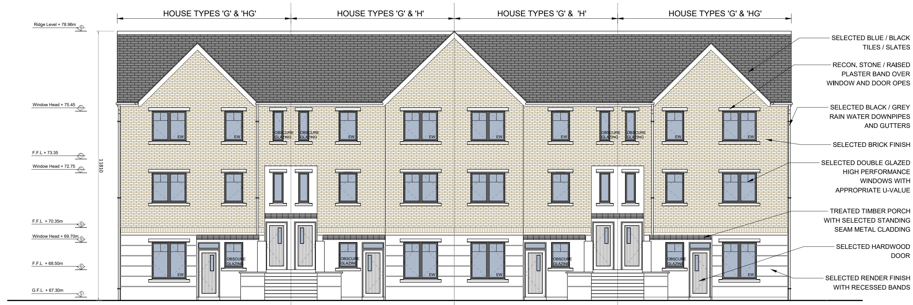
EAST ELEVATION - BLOCK J
